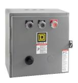
NEMA Starter, Type S, reversing, horizontal, Size 0, 18A, 5HP at 575VAC, 5kA SSCR, 3 phase, 3 pole, melting alloy overload, 120VAC coil, NEMA 1
